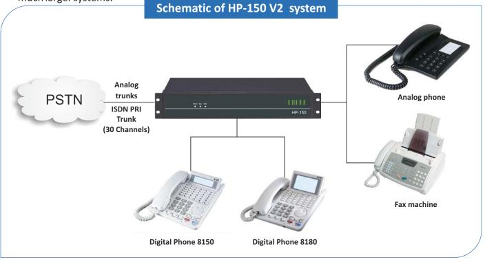
HP-150 V2 Communication System uses high speed CPU to handle high traffic loads. The system is flexible enough so that you can build the possible combination of trunks, analog phones and digital phones to suite your organizational requirement. The HP-150 V2 system also supports ISDN PRI (30 Ch.) interface which is a standard connectivity offered by telecom service providers for SMB customers.
